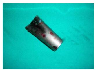
Fig. 4. Exploded lithium battery.
