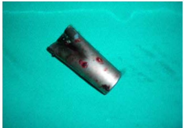
**Fig. 4.** Exploded lithium battery.
