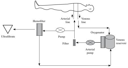
Figure 1. Ultrafiltration circuit during bypass.
