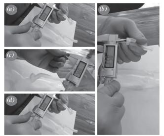
Figure 3. Manuel measurements of 3D printed physical models with a digital caliper. (a) Distal internal carotid artery inner diameter measured with a digital caliper. (b) Proximal internal carotid artery inner diameter measured with a digital caliper. (c) Carotid narrowing lumen diameter with a digital caliper. (d) Distal internal carotid artery inner lumen diameter measured with a digital caliper.
