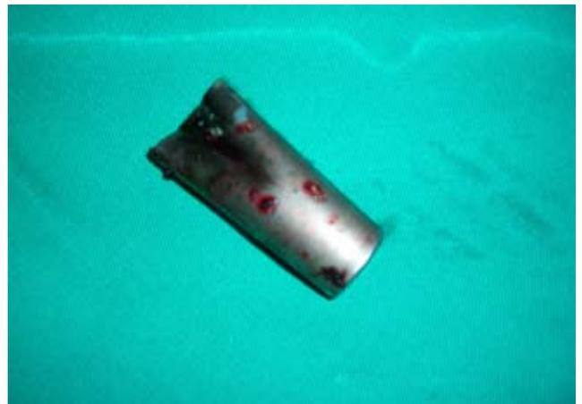
**Fig. 4.** Exploded lithium battery.
