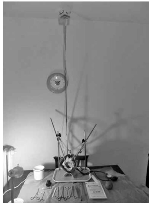
Figure 2. The surgical table with two atrial retractors mounted on two rods is shown. It features the capability of three-dimensional movement to stabilize the bovine heart. The aortic valve leaflets were removed, and the aorta was connected to a water-filled tubing system. The top of the water-filled column was open to the atmosphere, and the height of this column was approximately 170 cmH 2 O, which is equal to 125 mmHg.
